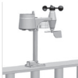
B. Mounting on the railing
